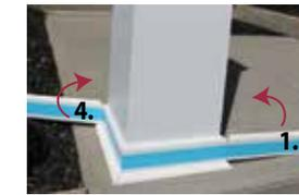
5 Unfold panel #1 and #4 into final position.
