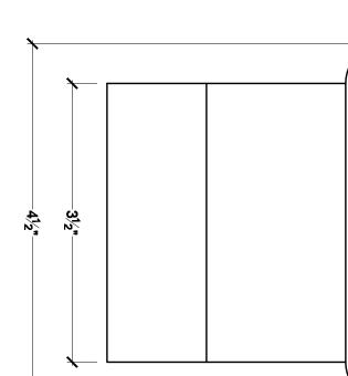
**OPERATIONS**1 INTERIOR OF BLOCK TO BE HOLLOW WITH OPEN BACK AND TOP
